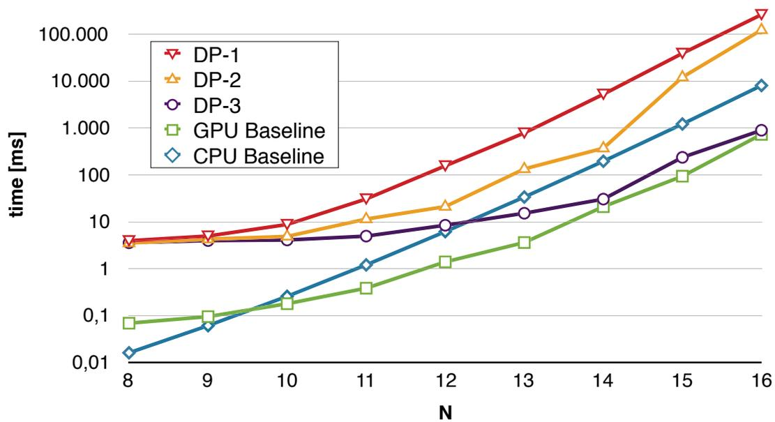
Figure 8: The approaches based on *Dynamic Parallelism* are not able to outperform the GPU reference [8], partially even the serial CPU reference [21]. Results are plotted on a log. scale.
