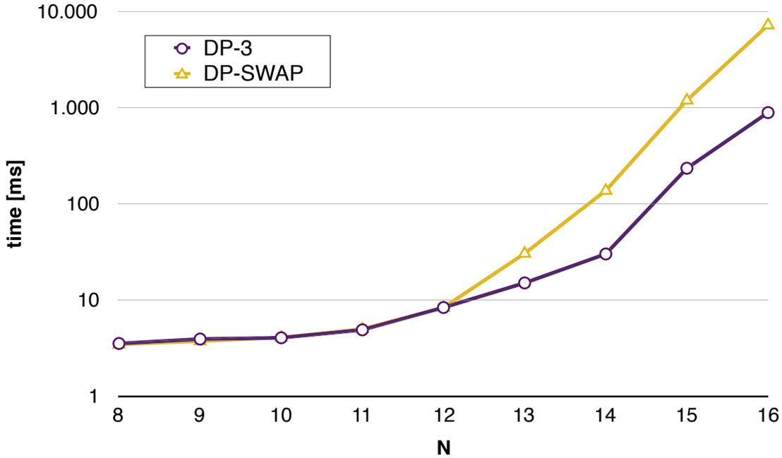
Figure 9: The swapping approach fails to gain speed-up over *DP-3* for all  $N$ . Increased shared memory consumption and static search depth are likely causes. Results are plotted on a log. scale.
