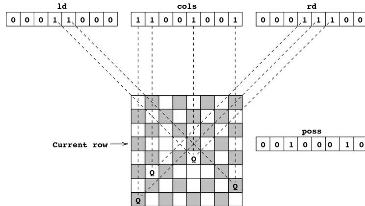
Figure 4: The chess-board can be efficiently represented using three bit masks. Bitwise operations can be applied to validate the current configuration. Image source: [18]
