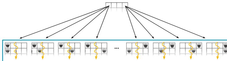
Figure 6: The improved version of *DP-1* processes multiple rows per grid and launches  $N^z$  threads, where  $z$  is the search depth.
