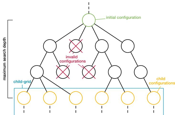
Figure 7: In *DP-2*, a thread traverses its subtree up to a maximum search depth. Valid configurations are passed to child grids.
