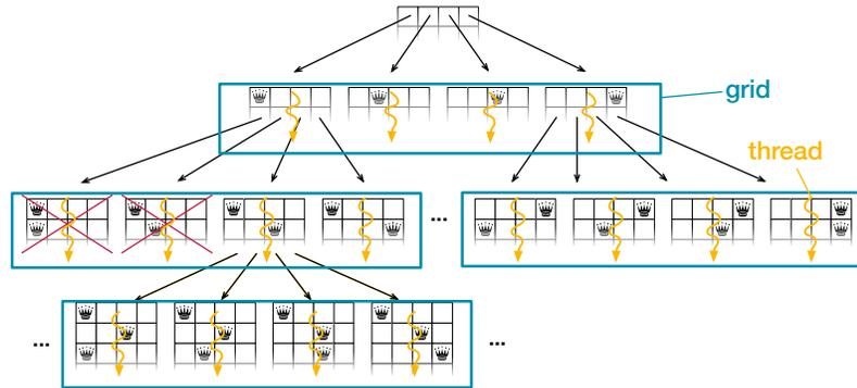
Figure 5: The first revision of *DP-1* launches one grid per row with one thread per field.
