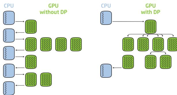
Figure 3: Without *Dynamic Parallelism* (DP), each step that influences the further control flow involves the CPU (left). Using *DP* (right), GPU kernels may launch child kernels by themselves.
