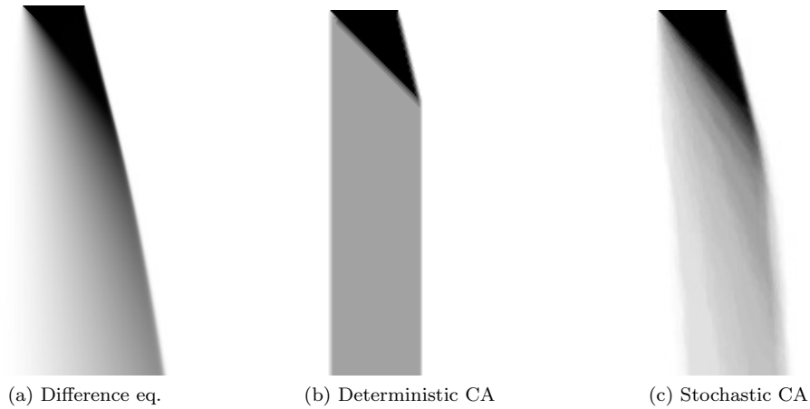
Figure 5: (a) Space–time plot of (2.8) with K_1 = 0.7 , K_2 = 0.14 , i = 0, \dots, 149 , and n = 0, \dots, 199 . The initial condition is given by 1 for i = 38, \dots, 74 ; 0 otherwise. The periodic boundary condition is applied. (b) Space–time diagram of deterministic Burgers' CA for K_1 = 0.7 , K_2 = 0.14 with k = 8 . (c) Average of 1000 space–time diagrams of stochastic Burgers' CA for K_1 = 0.7 , K_2 = 0.14 with k = 8 . (For (b) and (c), their initial configurations are given by k-1 if 38 \leq i < 75 ; 0 otherwise, and the periodic boundary condition is applied (space size: 150, time steps: 200).)
