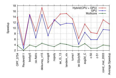
Figure 5: Displays the relative speedup of the Multi-core, GPU and Heterogeneous(CPU+GPU) w.r.t Sequential Approach
