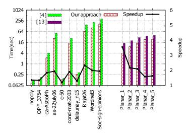
Figure 2: Figure displays the absolute time taken by our approach, labeled "Our Approach" compared to [4] for general graphs and [12] for planar graphs.
