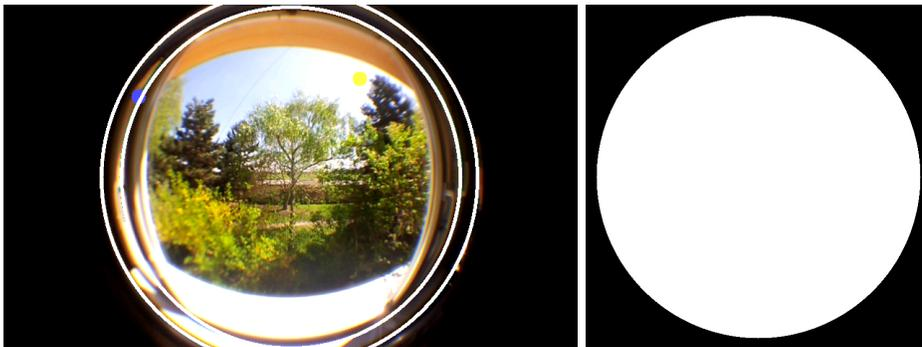
Figure 7: Clipping. Left: Clipping area is limited by inner circle while outer circle corresponds to the visible fish-eye area of 235° view. North direction is marked as a blue dot and the sun position is marked as a yellow dot. Right: The final clipping mask.
