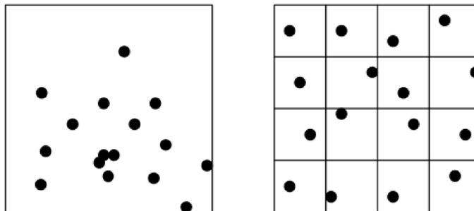
Figure 3: Calibration samples selected from the inside of the spherical panorama. Left: Random selection. Right: Evenly distributed random sample selection in a regular grid.
