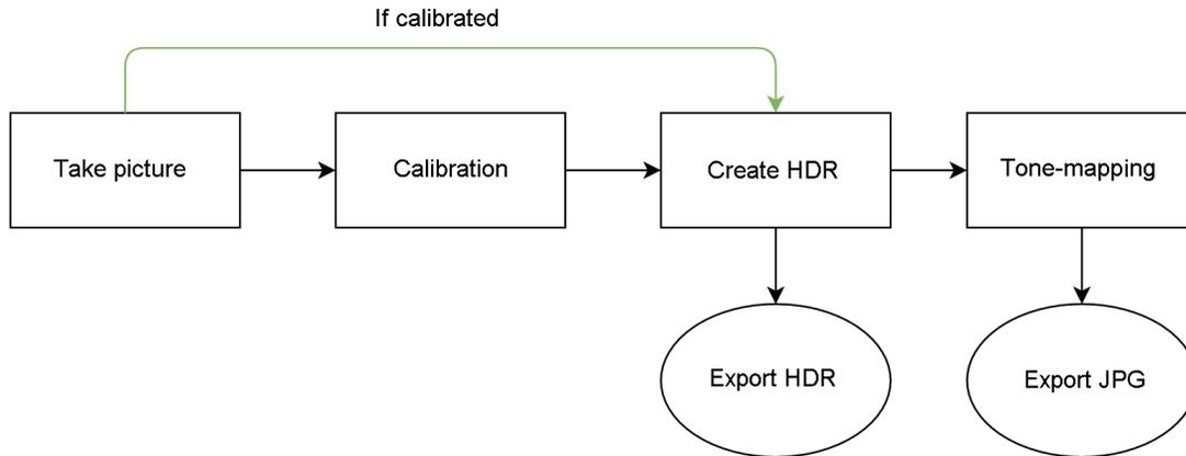
Figure 1: Pipeline for capturing the HDR panorama on a mobile device with few shots.
