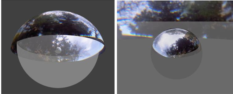
Figure 14: Applying captured HDR data as a radiance map to the 3D scene in the computer image synthesis. Left: Our panorama mapped to the spherical environment map. This environment map serves us as the light source in the form of the sky-dome. Right: Environment map applied to the spherical metallic object in the 3D scene.
