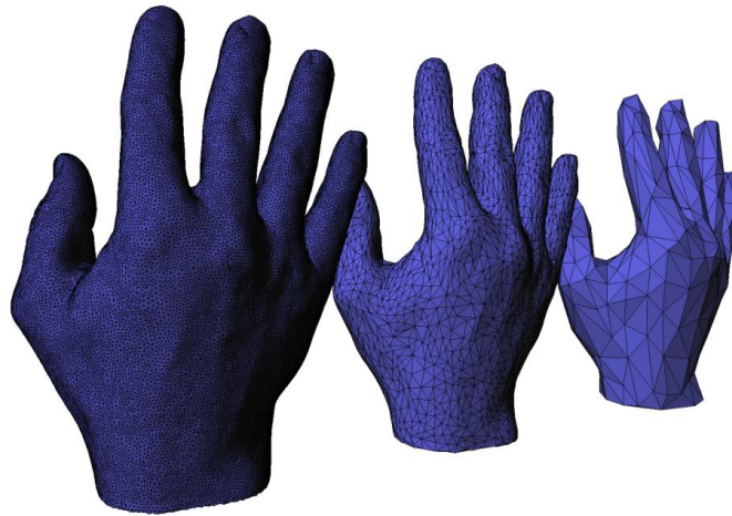
Figure 2: Surface mesh simplification algorithm applied to a mesh with different simplification levels [4].
