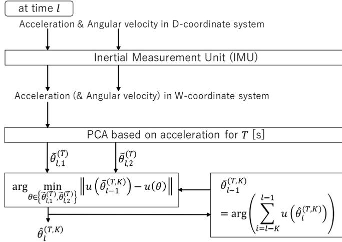
Figure 6: Flow of the proposed estimator
