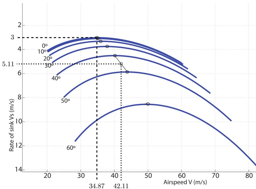
Figure 7: Hodographs of a Cessna 182 for various bank angles [4].
