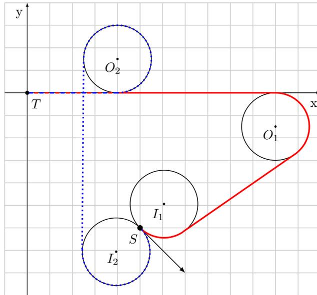
Figure 2: Schematic approach paths for LSLS and RSRS approaches.
