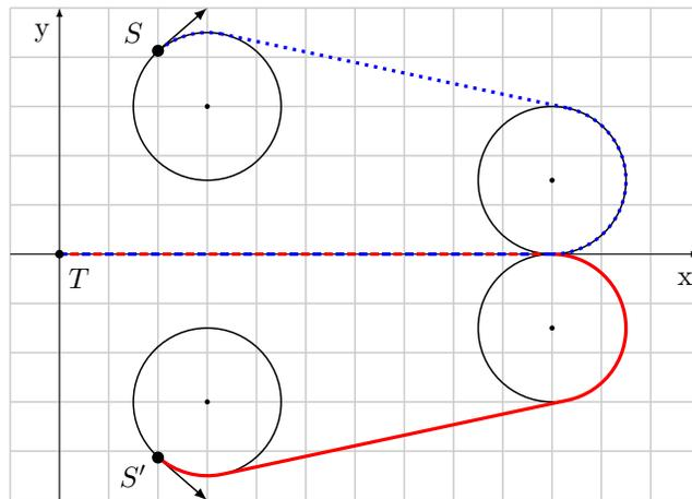
Figure 3: Mirroring at the  $x$ -axis and converting from RSRS-approach to LSLS-approach.
