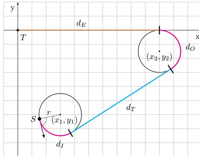
Figure 4: Approach segmentation for the LSLS approach.
