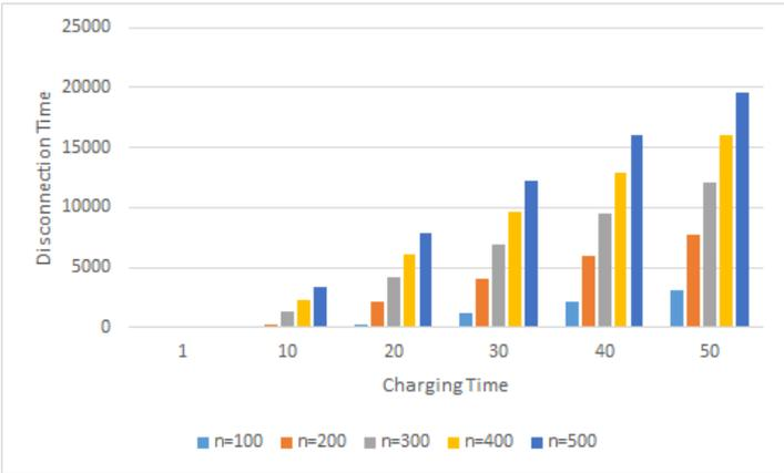
Figure 5: Effect of Charging Time  $\rho$  on Disconnection Time;  $\Delta=2000, d=1$
