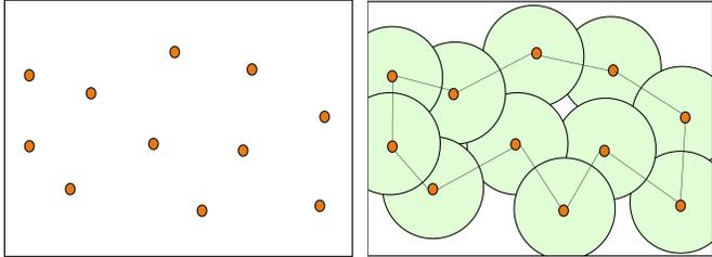
Figure 1: a) A deployed sensor network. b) A cyclic order  $\pi$  of the nodes.
