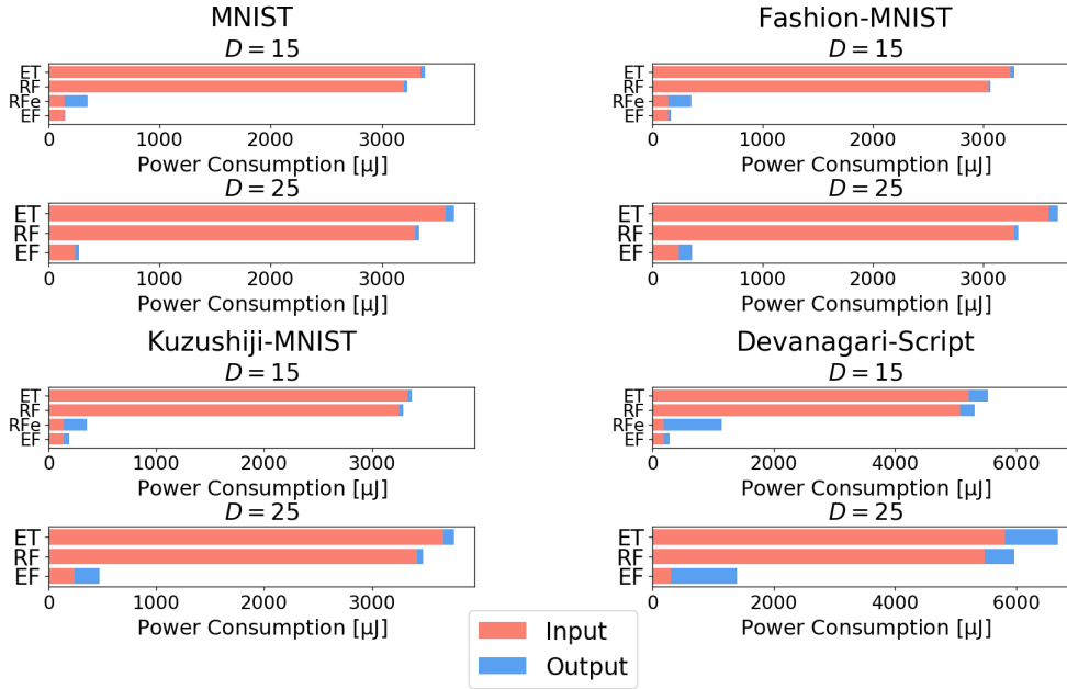
Figure 6: Power consumption comparison between MNIST, Fashion-MNIST, Kuzushiji-MNIST, Devanagari-Script. ET, RF, RFe, and EF represent extraTrees, randomForest, rFerns, and ExtraFerns. In each graph, red bars and blue bars show the power consumption required to load training data from DRAM and write a trained model back to it. From the result, we can confirm that ExtraFerns requires minimal power consumption in every condition.
