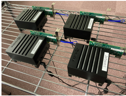
(a) An embedded GPUs cluster consisting of four Jetson Xaviers
