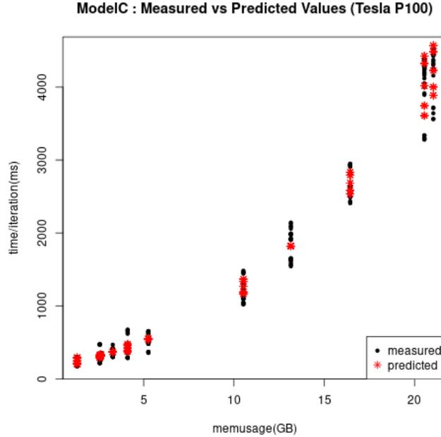
Figure 4: Model C:Predicted and Measured Responses (Tesla P100)
