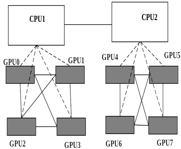
Figure 2: Device Architecture
