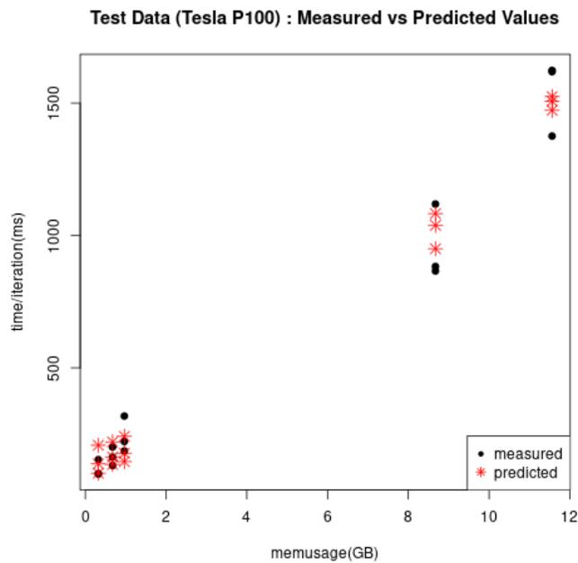
Figure 5: Model Test: Predicted and Measured Responses (Tesla P100)
