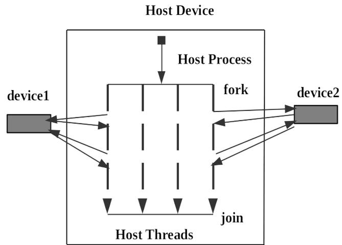
Figure 1: Hybrid Programming Model
