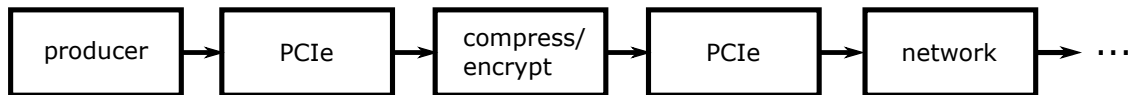
Figure 7: Example flow graph for FPGA accelerated compression/encryption using a traditional FPGA interconnection.
