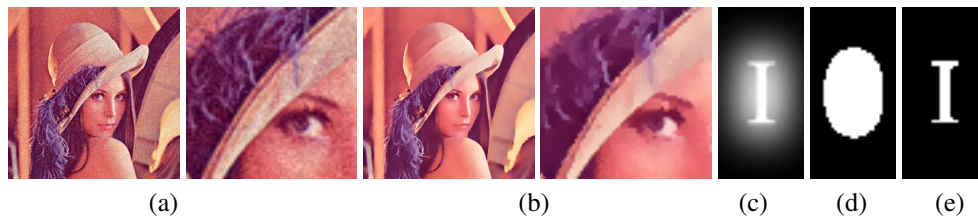
Figure 2: Image processing examples using VCAT. Since biomedical images are often corrupted with noise, denoising is important for processing such images. The image (a) was corrupted with additive Gaussian noise, artificially. The image (b) demonstrates a result of denoising with edge-preservation, which was obtained by applying Domain Transformations (DT) [24] to the corrupted input image (a). Biomedical images may also consist of a gradation of background intensity due to their imaging conditions. The image (c) mimics a such condition, and applying the Otsu method [48] to (c) gave a undesired segmentation result (d). Employing Top-Hat transformation [26] prior to the Otsu method provided a better segmentation result (e).
